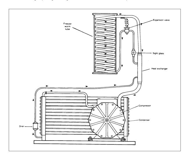
As it evaporates, it absorbs heat from the evaporator and whatever is in contact with it (such as the water inside it).
