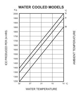
NOTE. Daily ice capacity is directly related to condenser air and water inlet temperature, water temperature to make ice - and age of machine.
