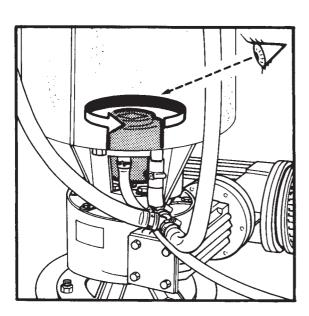
2. Press unit lighted switch to ON. Unit will start operating. Verify immediately if auger drive motor turns the auger (coupling) in counterclockwise direction.
